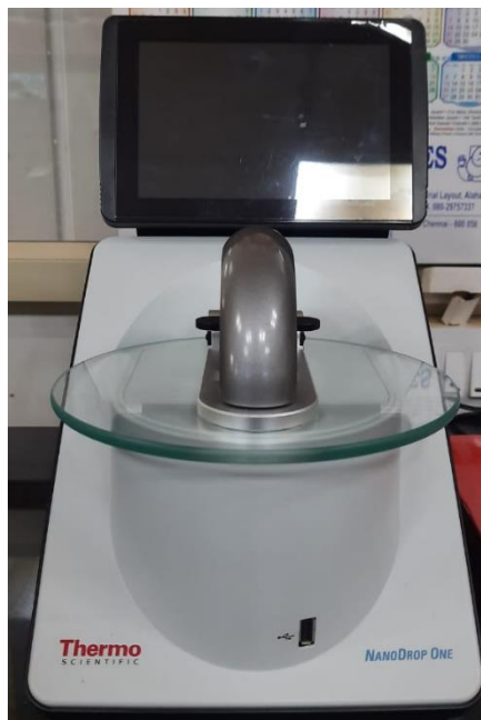
Figure:-.11 Nanodrop spectrophotometer from Thermo Scientific measures the purity of nucleic acids.
