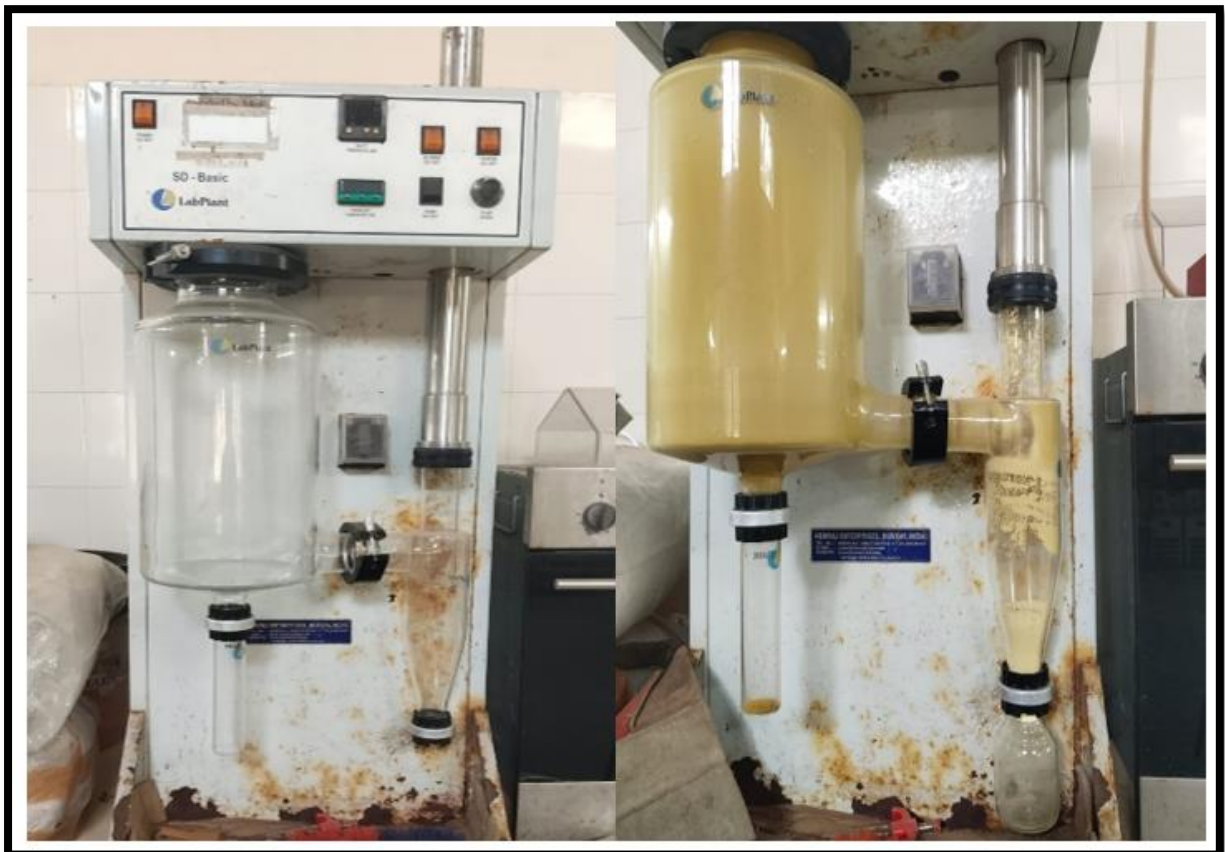
Fig 19: Spray drying machine and Kashaya extract making of Kshamatva churna
