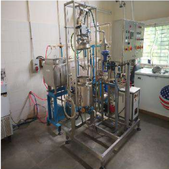
Single batch Evaporator
