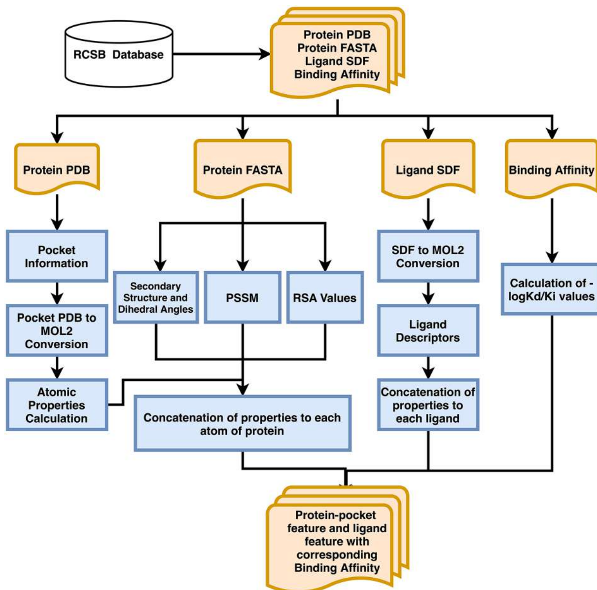
Figure 1. Feature extraction pipeline. PSSM indicates Position-Specific Scoring Matrix.
